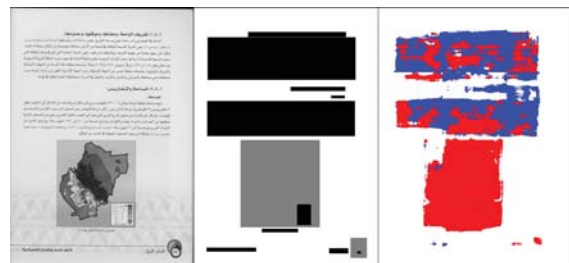
Fig. 4. One of the low resolution samples in set A and its poor segmentation using the FCN trained on samples with higher resolution.
