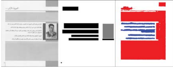
Fig. 6. Test sample (left) contains complete non-text zones which is not annotated (middle) but recognized by FCN (right).
