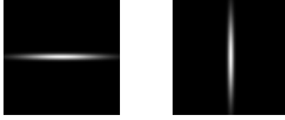
Fig. 4: Narrow anisotropic Gaussians used for masking ( \sigma_x = 1 ; for visualization, \sigma_y = 15 is shown). Left: horizontal ( \theta = 0 ). Right: vertical ( \theta = \pi/2 ).
