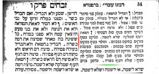
Fig. 5: Illustration of separator region preservation in a document with an L-shaped layout. On vertical separator regions, no matter how narrow they are, a narrow vertical Gaussian (red) will lead to a high response. Similarly, on horizontal separator regions, no matter how narrow they are, a narrow horizontal Gaussian (green) will lead to a high response.
