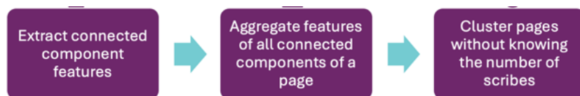
Fig. 9. Overview of the proposed pipeline: connected component feature extraction, page-level feature aggregation, and unsupervised clustering of page images.
