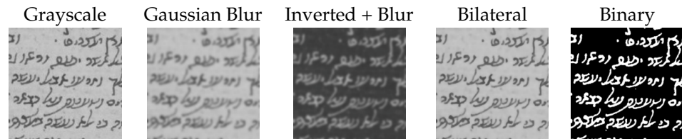
Figure 5. Example of the input patch types we experimented with.
