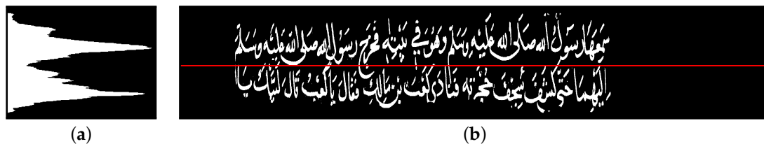
Figure 6. Splitting combined lines: (a) the horizontal profile of an image patch, and (b) the mask is split at the minima closest to the center of the mask. The split line is shown in red.
